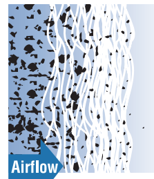
"Progressive Density" construction prevents faceloading, and increases arrestance and dust holding capacity.
