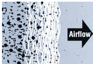
Progressive Density Media Construction
